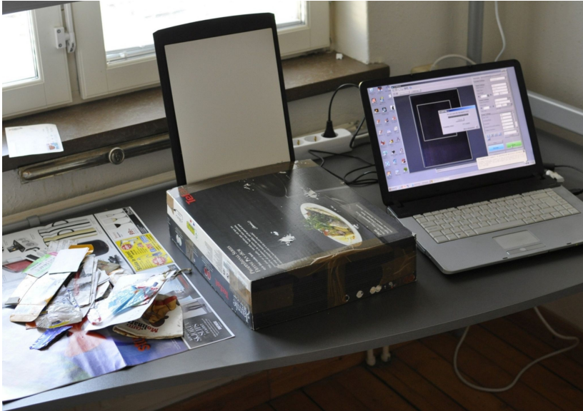
Fig.128 Picture showing a set up I adopted to scan trash. On the left the trash is put on a newspaper to collect all the dirt that might fall from it and the scanner is covered with a box so as to keep the scanning plate dark. If I scan at night the cardboard is not used and the light is switched on and off. In this picture my bed is just above the desk.
