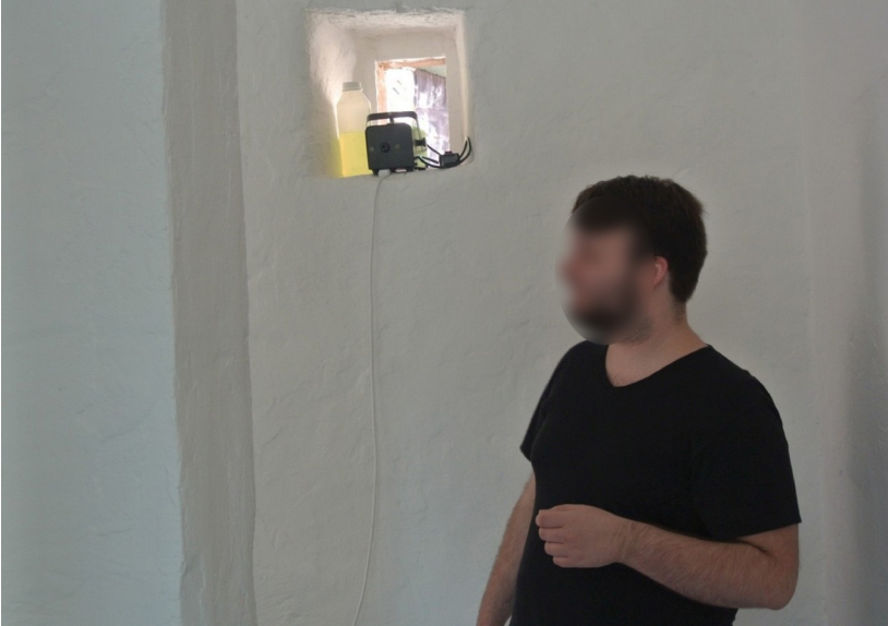
Fig.178 Picture showing a visitor of my installation in the alps where a smoke machine was placed to reproduce the air quality I keep track of. The smoke machine button is replaced with a relay controlled by a microprocessor reproducing my data. This can be also reproduced by the visitors who can press the button according to my record.
